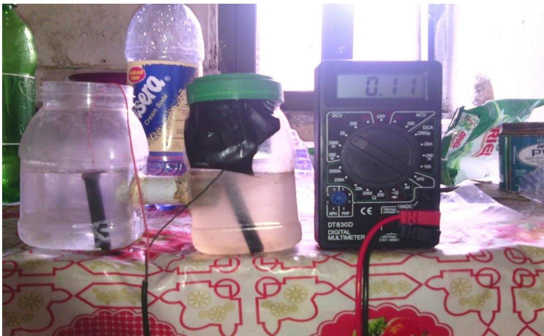
PLATE 2: photograph of double chambered waste water microbial fuel cell
