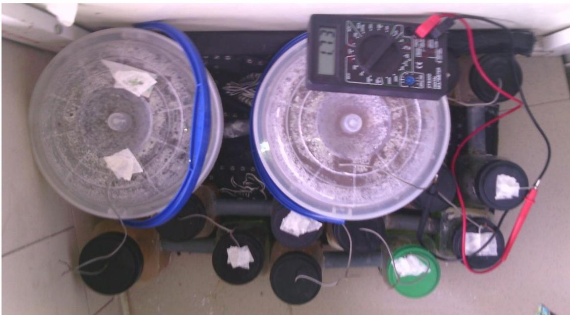
**PLATE 3: Stacked wastewater microbial fuel cell**
