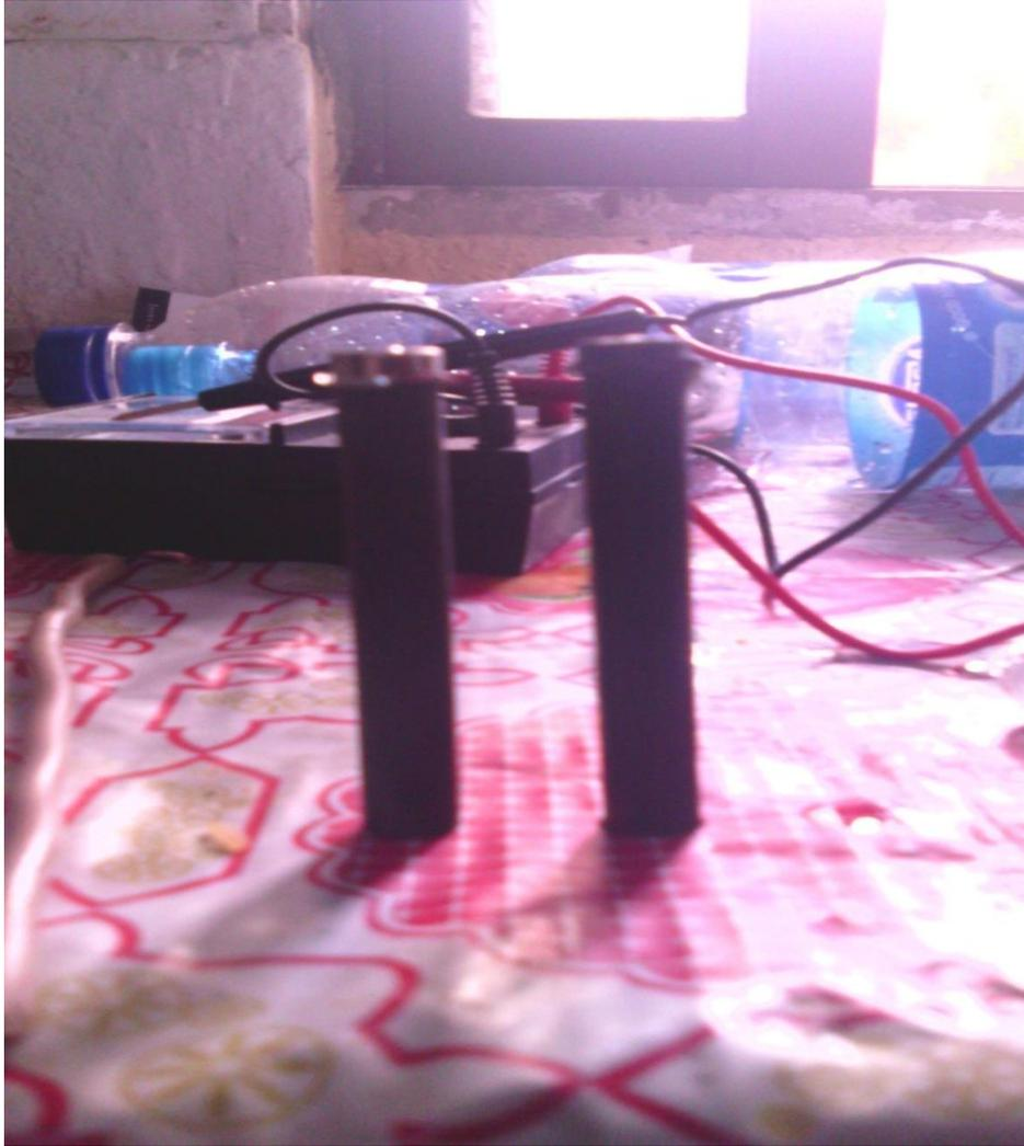
PLATE 1: photograph of the graphite electrodes
